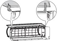
3. Press 4 places on the intake grille to close it completely.
