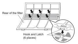
Replace the air filters and close the intake grille. Refer to steps 4 ~ 5 of "Cleaning air filter".
